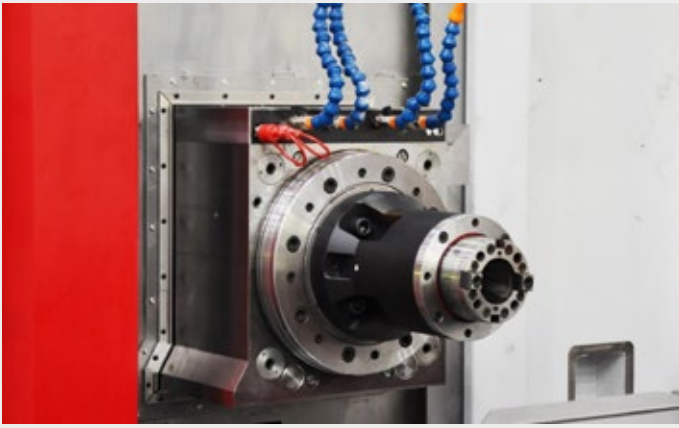
HEADSTOCK WITH SPINDLE TRAVEL 1000 MM
