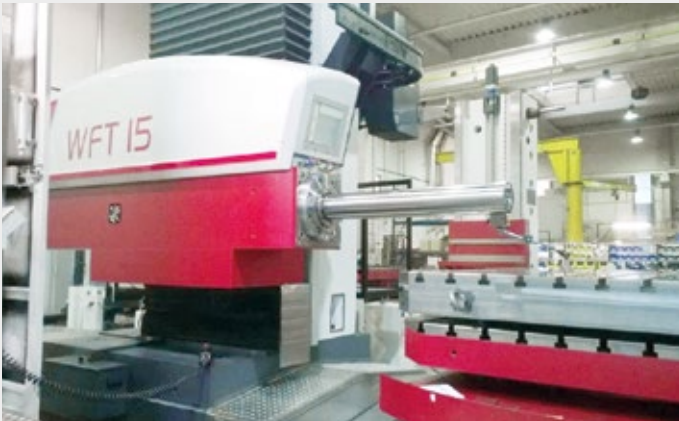
HEADSTOCK WITH SPINDLE TRAVEL 1000 MM
